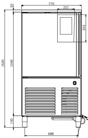
AUSGANG STROMKABEL 380-415 V3N / 50 Hz
