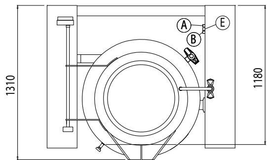
**A** Allacciamento acqua calda - Hot water inlet pipe - Raccordement eau chaude - Warmwasseranschluss      3/4"
